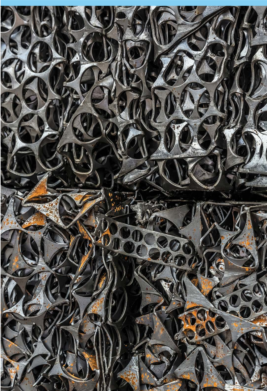
Scrap iron used in SP process.
