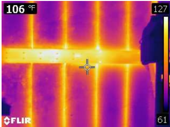
The seams of oven doors are far less insulated than the rest of the door.
