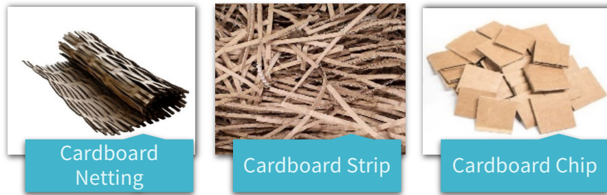
Figure 4 - The different product types of cardboard after it is put through a shredder or perforator.
